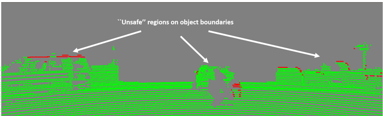
(c) The safe depth image of the reconstructed keyframe view.
