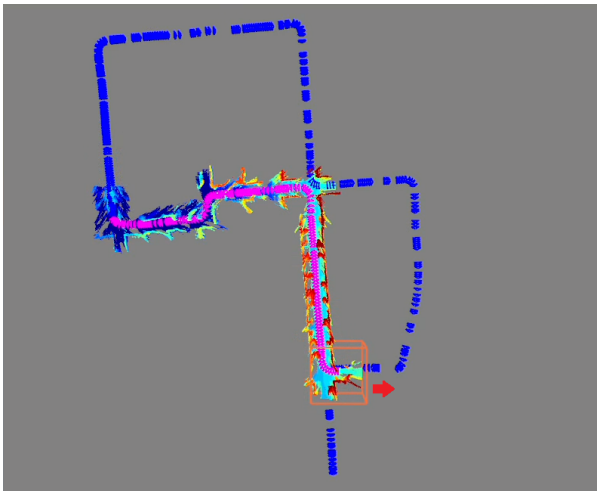
(d) The top-down view of the reconstructed local dense map before loops.
