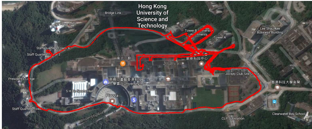
Figure 29: The estimated trajectory (shown in red) on a long walk around the HKUST university campus. We plot it on the top of the Google map of the campus. The path is almost aligned with the map.
